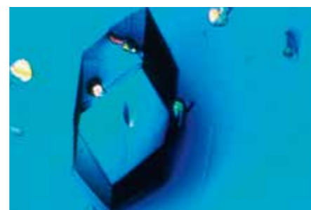
(B) Crystals of apocrusacyanin C1 from lobster carapace optimised using an oil barrier in hanging drop [5]
